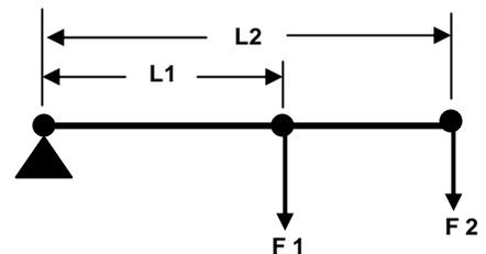
The Cylinder Force “F1” is calculated by multiplying the Regulated Pressure “P” times the total Effective Area of the cylinder(s).
